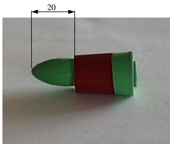
**Figure 2.4.** Bung with balloon fitted to form diaphragm-piston. Note the insulation tape wrapped around the narrow end of the bung to prevent radial expansion of the balloon.
