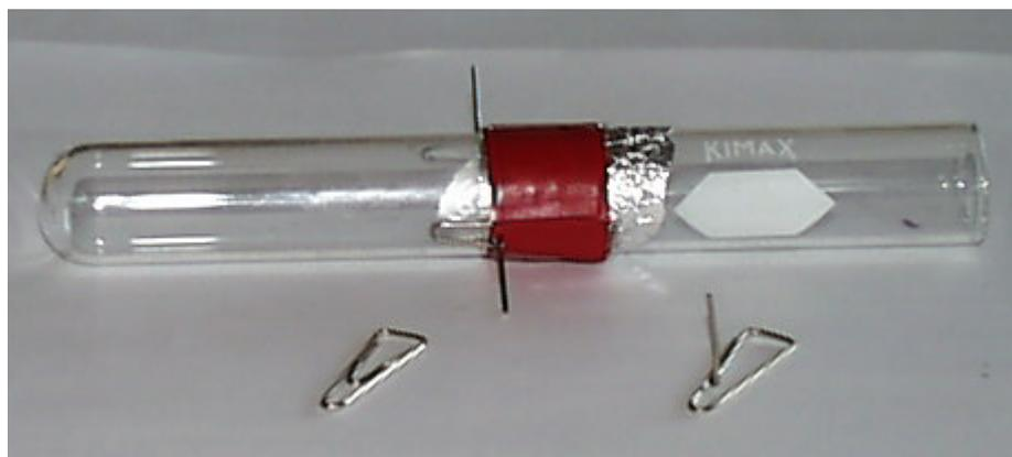
**Figure 2.2.** Paper clips before (left) and after (right) modification. Attachment of paperclips to the test-tube (background).
