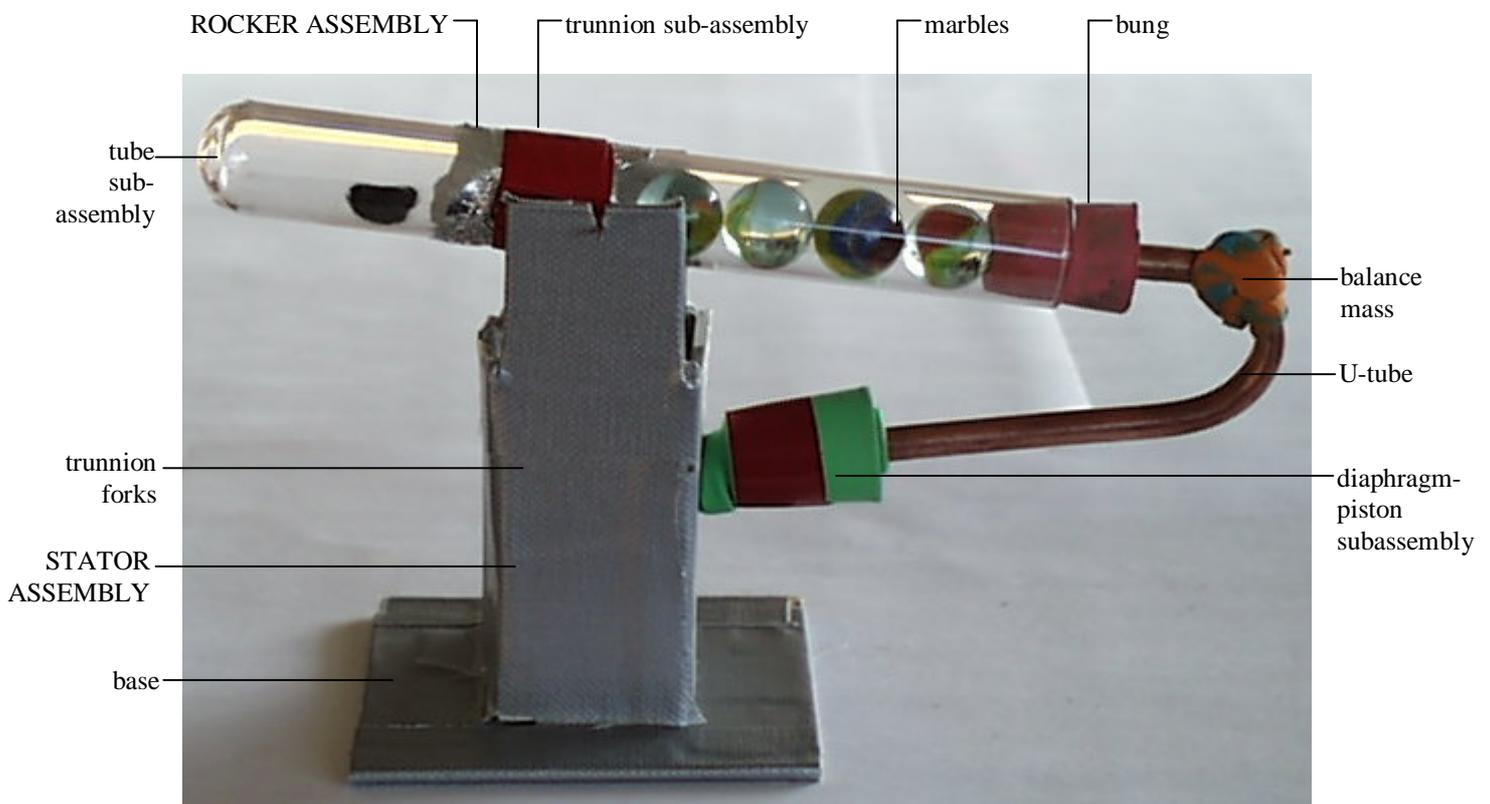
**Figure A.** The test-tube Stirling-cycle engine.
