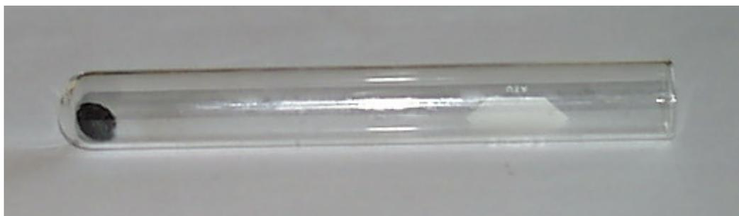
**Figure 2.3.** Steel wool in the end of the test-tube.
